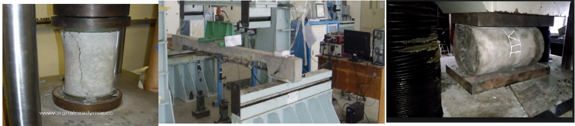
Uji Tekan (ASTM C39)
